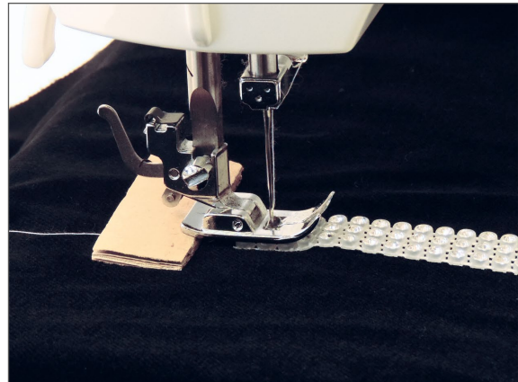
The presser foot lies flat due to the height compensator.
