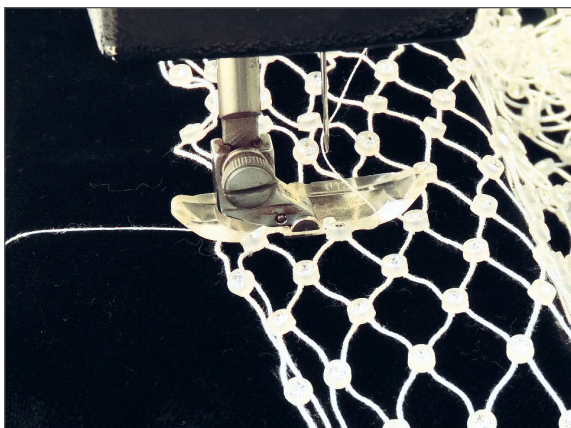
Use a narrow „zipper“ foot when appropriate due to the applied product.
